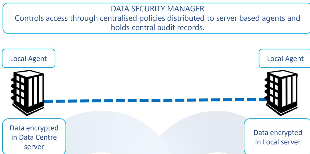
The encryption agent are inserted above the file system logical volume layers and control access to protected data, referring to the policies set in the Data Security Manager. The agents perform the encryption, decryption and access control work locally on the system that is accessing the data at rest in storage. This enables encryption to be distributed within the data centre and out to remote sites while being centrally managed.
